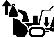
Weight Transfer Depress Pedal To Disengage
