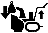
Weight Transfer Lift Handle To Engage
