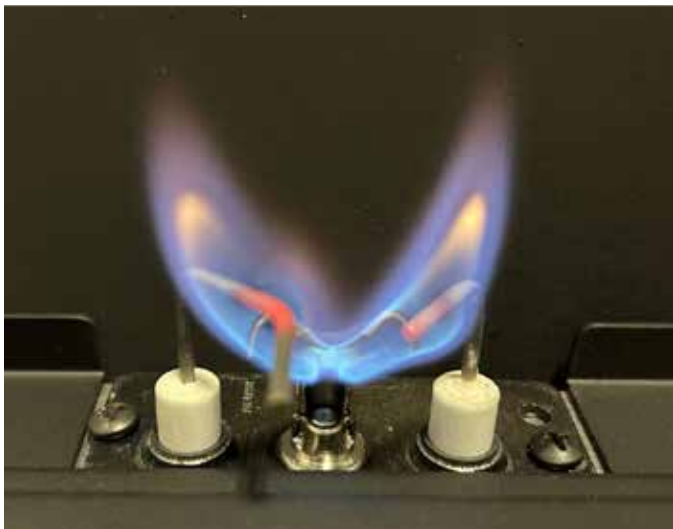
Figure 7.8 IPI Pilot Flame
