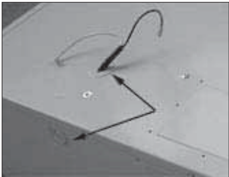
3. If using a cable lock, pry open the desired electrical knockout either on top or back of hood. Feed the wires through the cable lock. Some local codes require the use of a cable lock, check your local codes.
