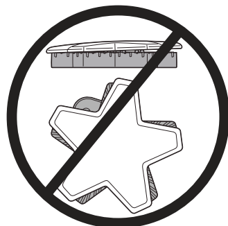
Incorrect burner cap
