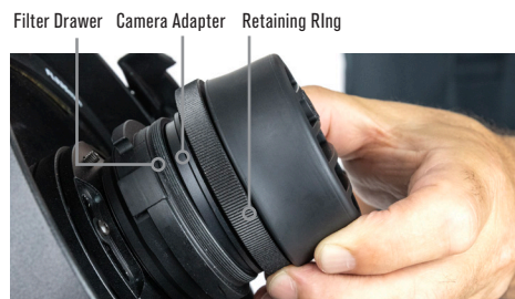
Fig. 8: Seat the camera adapter onto the exposed filter drawer, then tighten the retaining ring.
