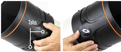
Fig. 1: Remove the lens shade by pressing down on the two tabs while pushing upwards under the Origin logo.
