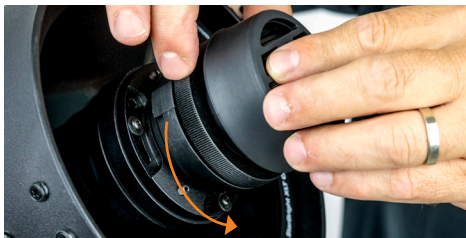
Fig. 2: To remove the Origin-178C camera from Origin, first unthread the retaining ring.
