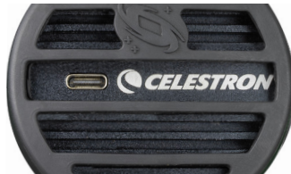
Fig. 6: Install the rubber cover on the Origin-678C so it appears as shown.
