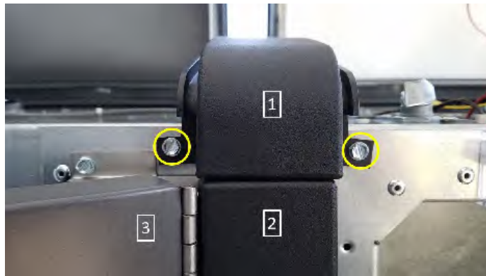
Tombstone [1] and Front Fascia Strip [2] secured by screws (circled)
