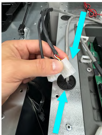
Feed Companion Extension Cable (ELCBB60019) through Grommet
