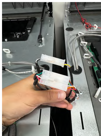
Plug into Companion Sensor Cable (ELCBB50010)
