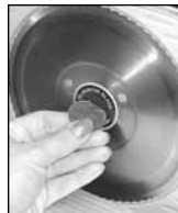
Figure 7. Turn the screw clockwise for blade removal.
