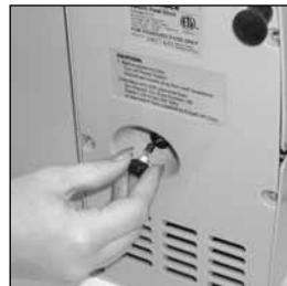
Figure 10. Replacing the fuse located underneath motor housing.
