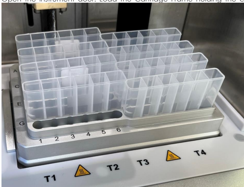
Figure 47: Cartridge frame loaded with eight reagent cartridges on the workdeck.
