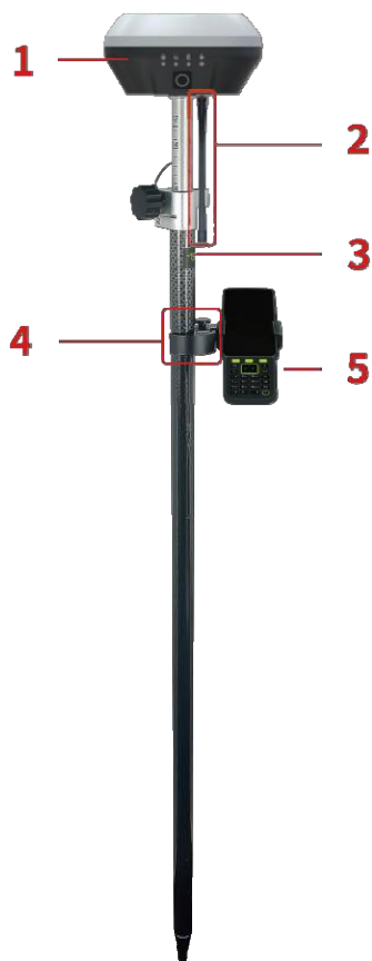
Figure 1.2 TS21 as a Rover – Internal Radio
