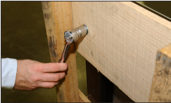
Removing skid from bottom of cabinet.
