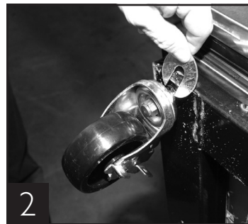
2 For leveling, insert the shim between castor and frame rail.
