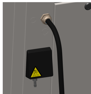
Figure 8: Hose connection for compressed air
