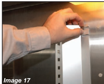
Pilaster Installation Two and Three Door Models (Middle of Wall in Rear of Cabinet)
