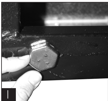
Back out leg levelers by hand, or with adjustable wrench.
