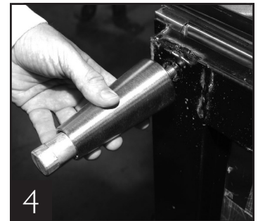
4 Thread leg into cabinet bottom frame rail.
