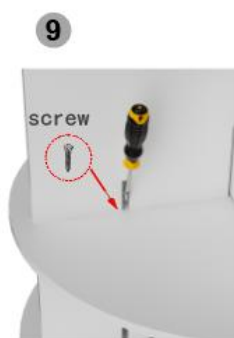
Each layer of square vertical hole screw reinforcement
