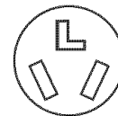
3-wire receptacle (10-30R)
