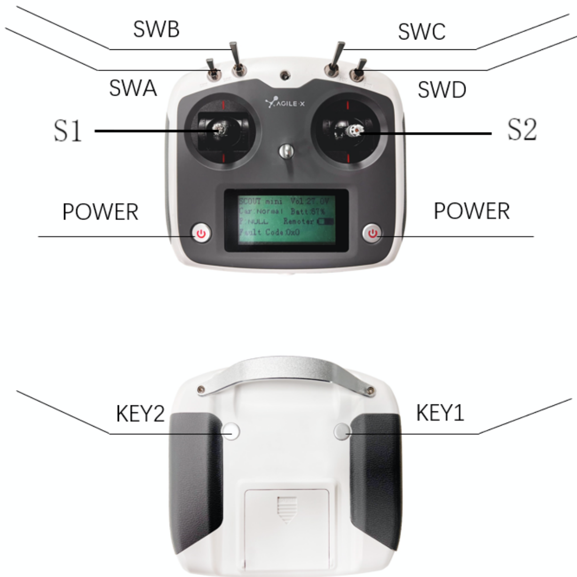
Figure 2.3 Schematic diagram of FS remote control buttons
