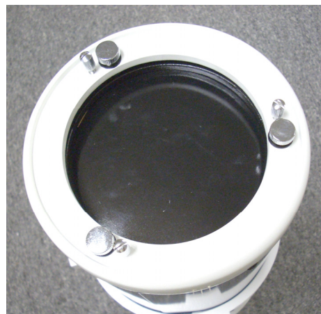
Figure 7-6 Primary mirror. Large thumbscrews are for collimation and small thumbscrews are for locking the mirror in place.
