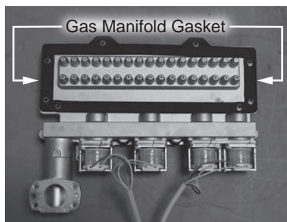
Figure 128 - Replacing gas manifold gasket
