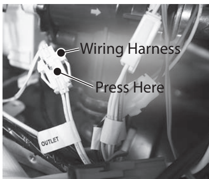
Figure 73 - Wiring harness location
