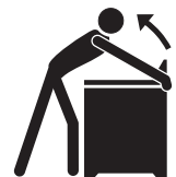
Range leveling leg
