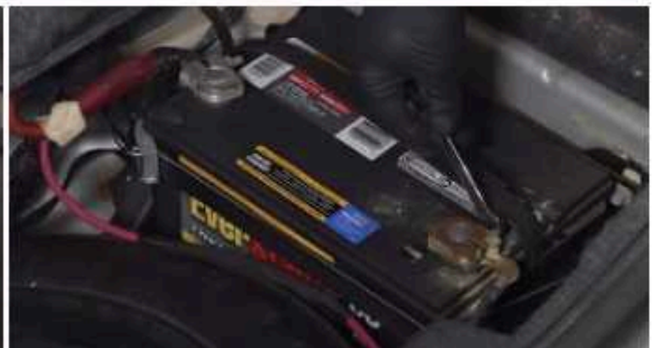
Disconnect the battery
