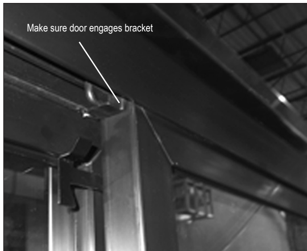
Figure 14: Removing/Installing Sliding Door
