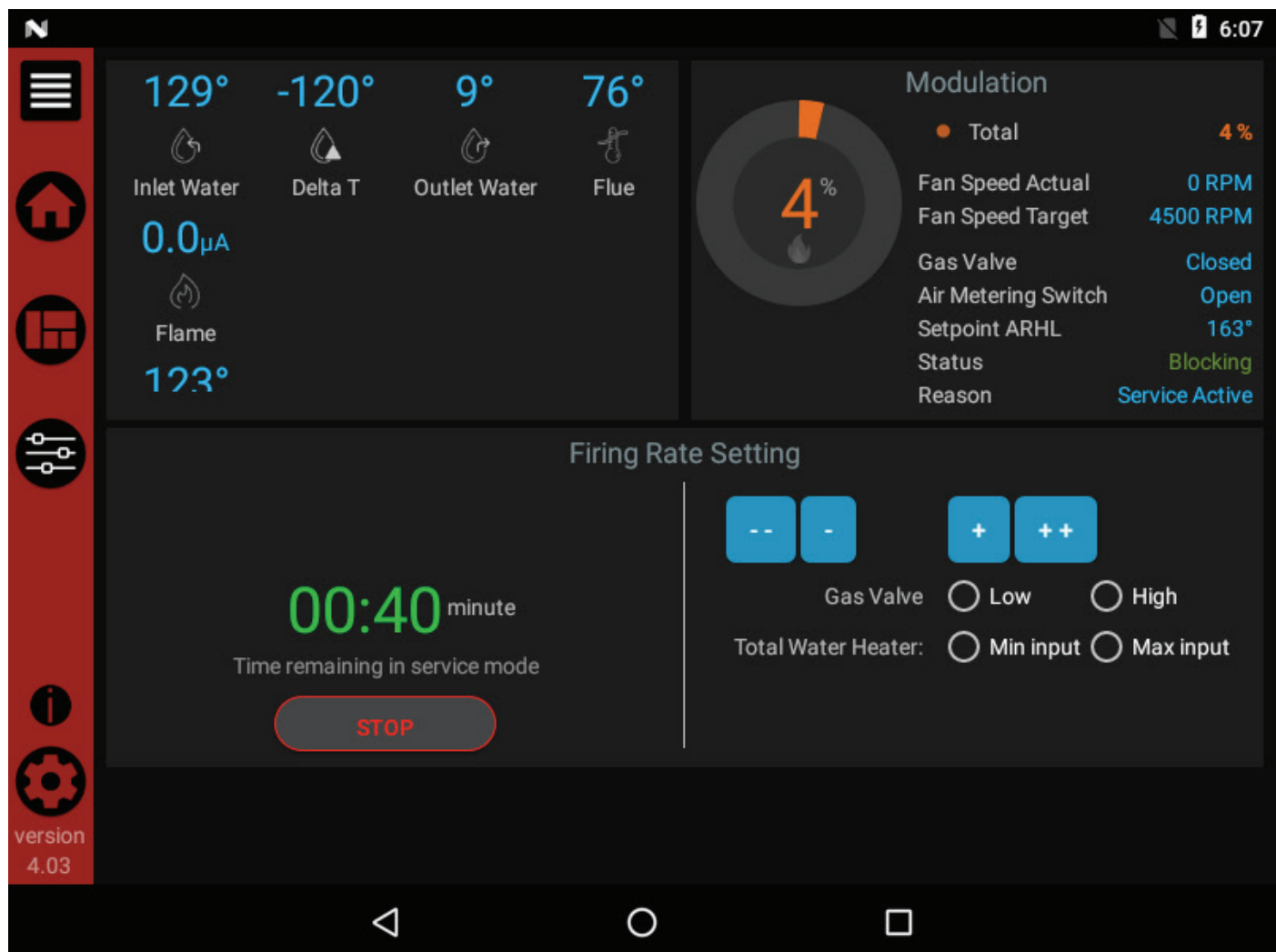
Figure 10-2 Service Maintenance Screen
