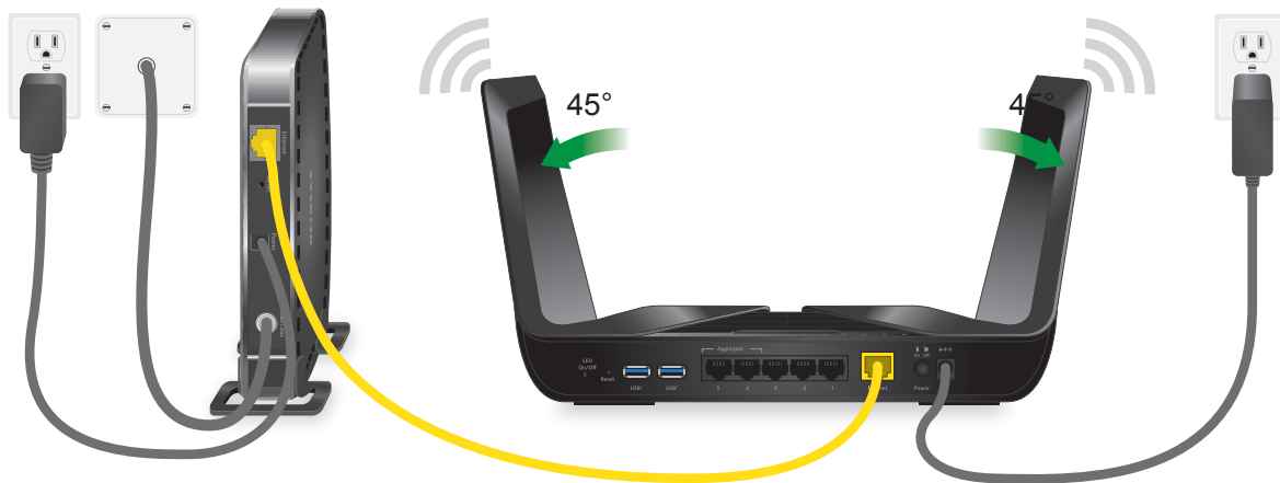
Figure 6. Cable your router
