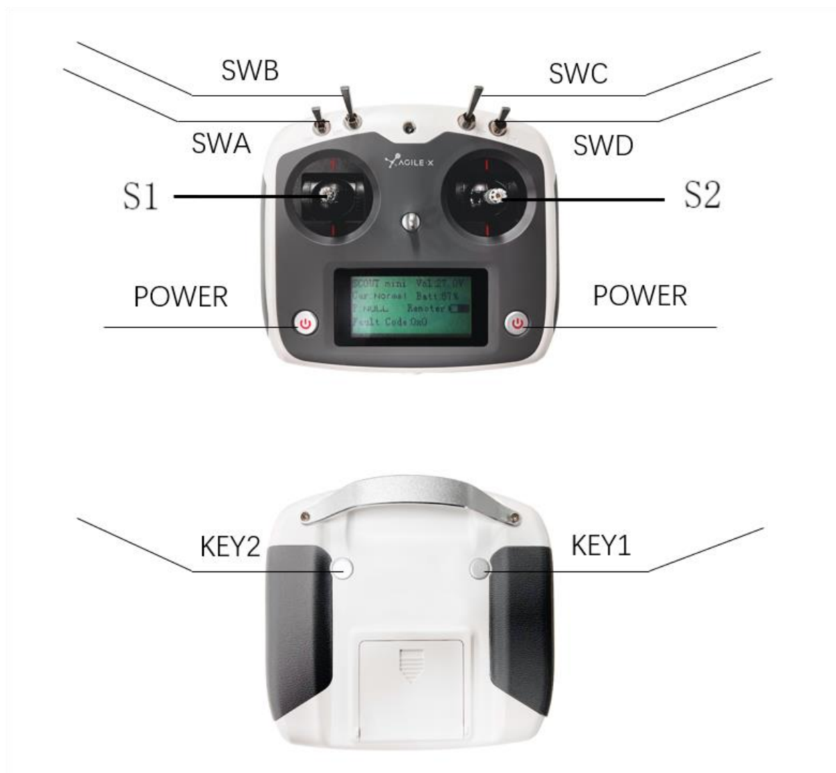
Figure 2.5 Schematic diagram of FS controller buttons
