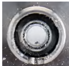
Top of the contaminated connecting bar
