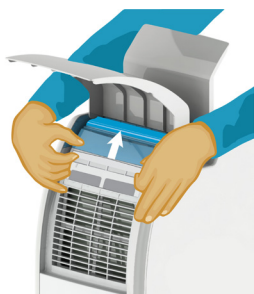
RETURN AIR INLET FILTER
