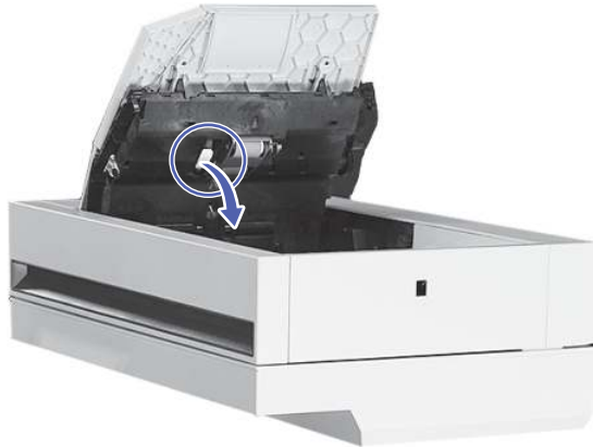
Figure 9-12 Release the blue locking arm
