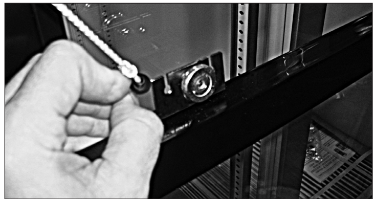
Fig. 6. Slide the the black tab holding the door cord out the back
