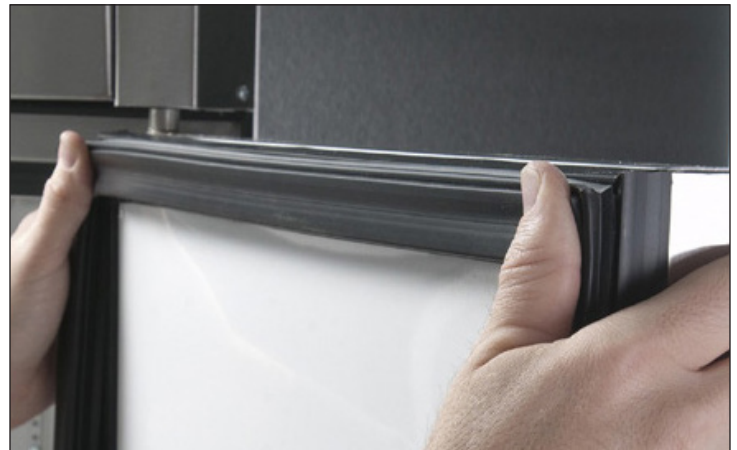
Fig. 4. It is common to see silicone pushed out of track around the gasket. This is how you know enough silicone was used.
