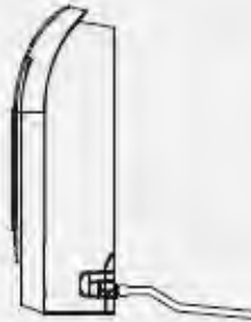
Install the drain pipe
