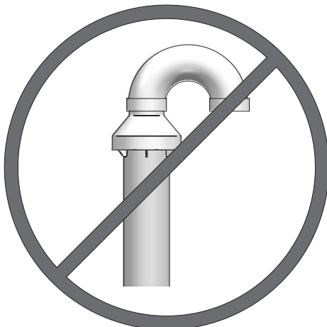
Figure 5-5 Do Not Install U-Bend to Rain Cap
