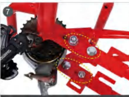
7. All screws and nuts are tightened.
