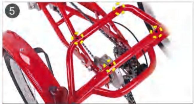
5. Four holes for fixing basket.
