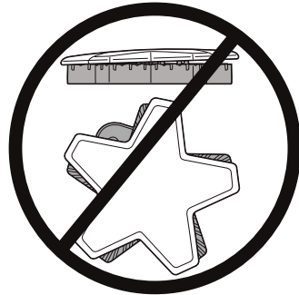
Incorrect burner cap
