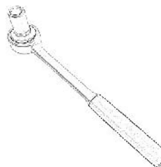
SOCKET WRENCH W/ 1/2" SOCKET
