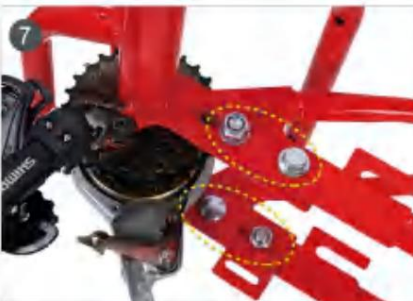
7. All screws and nuts are tightened.
