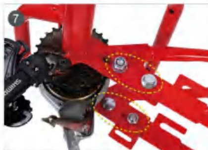
7. All screws and nuts are tightened.
