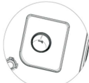
3. Rotate the lifting cup till the lifting cup slot and water tank buckle are fastened.
