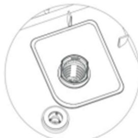
2. Properly install the flat strainer according to the shape corresponding to the flat strainer.
