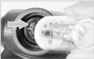
2. Match the red dot on the base of the flash tube with the red dot in the Tube Socket (4). Push the flash tube in until it is securely seated into the socket.
