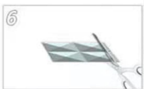
Step 6: Cut the panel to suit the wall corner.
