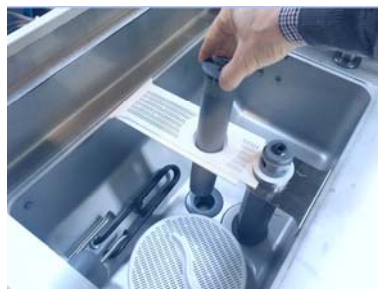
Remove the overflow pipe
