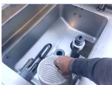
Insert the filter pump suction
