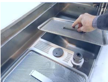
Remove the filters tank
