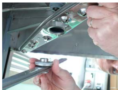
Remove the reel clearing top
