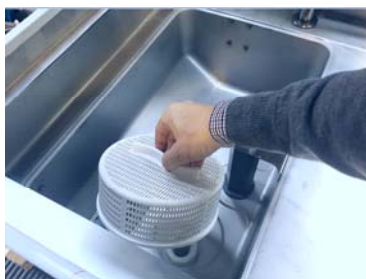
Remove the filter suction pump
