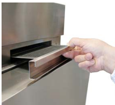
Clean the filter of the steam condenser that is placed in the upper part of the hood;
