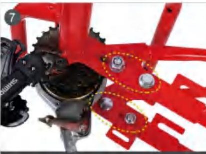
7. All screws and nuts are tightened.
