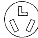
3-wire receptacle (10-30R)
