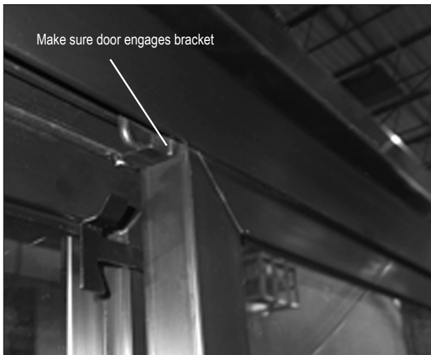
Figure 14: Removing/Installing Sliding Door
