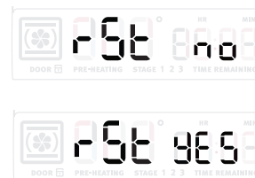
Figure 29: Display showing the options to reset to default (rSt yes) or to reject resetting to default (rSt no)
