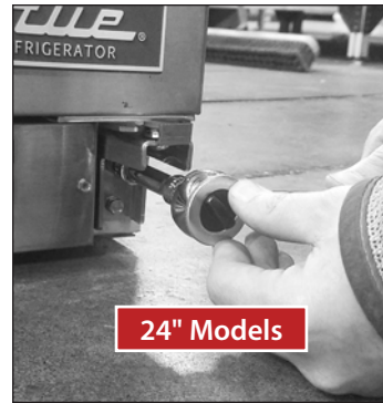
Fig. 1. The 24 and 27 models use different lower hinges.
