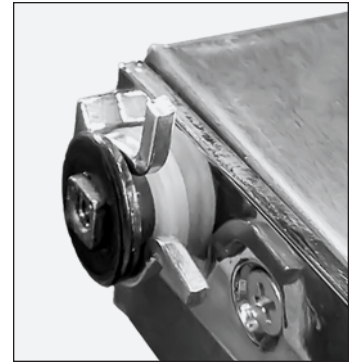
Fig. 7. Keep the washers in their original order.
