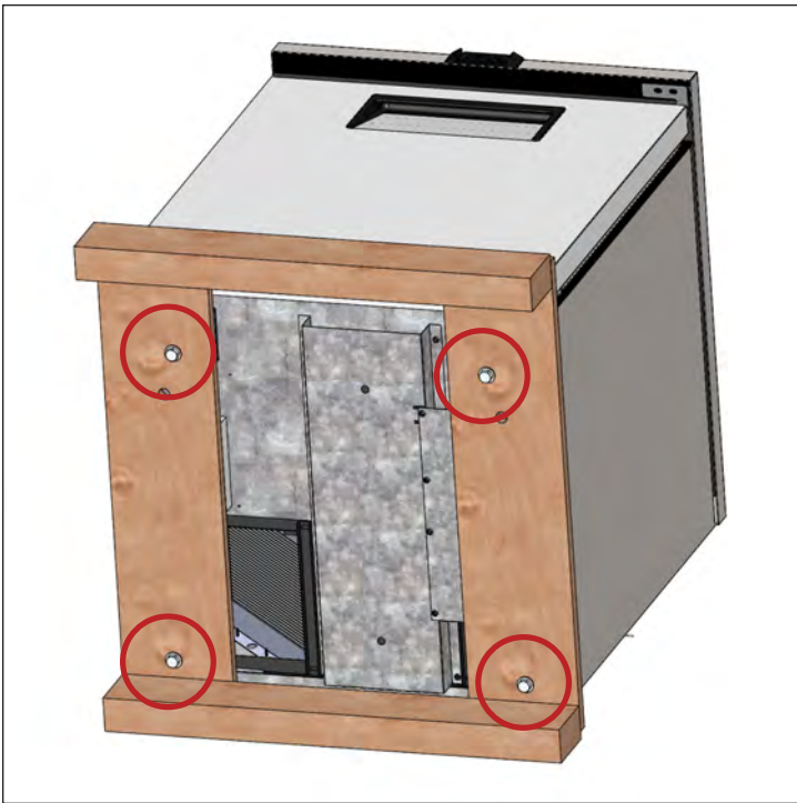
Fig. 3. Remove all shipping bolts.
