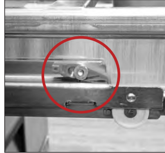
Fig. 5. Drawer retainer location. Retainer is engaged.
