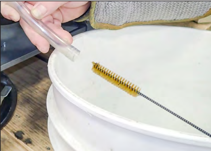
Fig. 2. Catch trapped liquid in a large container.
