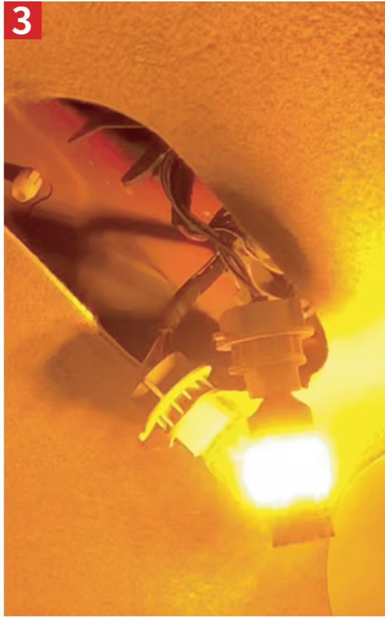
Test If the LED Bulb Light Up
