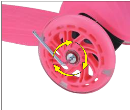
Right Wheel: Turn the Allen key clockwise to loosen the screw.
