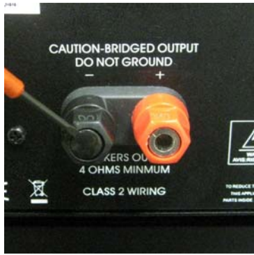
Removing the binding post insulators
