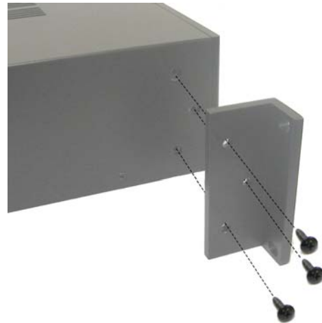
Installing Front Rack Ears
