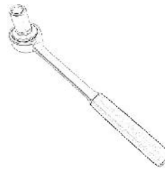
SOCKET WRENCH W/ 1/2" SOCKET
