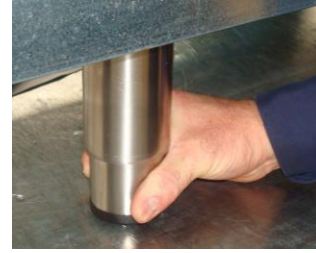
Adjust the legs to level the unit
