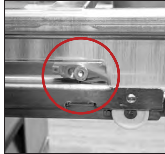
Fig. 5. Drawer retainer location. Retainer is engaged.
